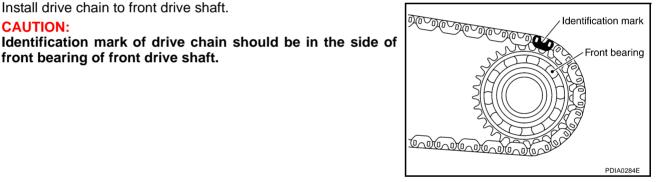
4. Install drive chain to mainshaft, and then install tap front drive shaft with plastic hammer. Press-fit rear bearing of front drive shaft to rear case.
