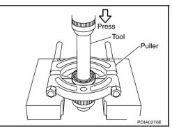
Remove front drive shaft rear bearing, using drift and puller.
