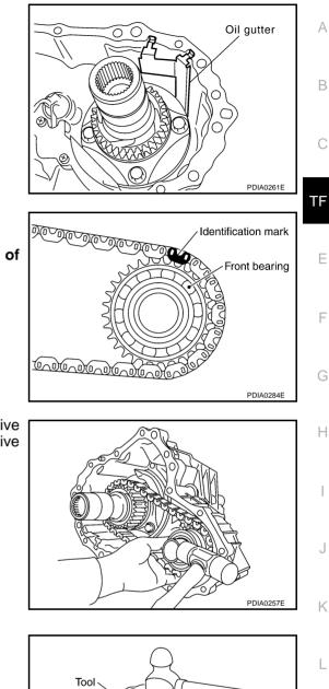
12. Install drive chain to front drive shaft.
