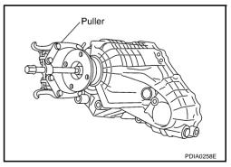
Remove companion flange, using a puller.
